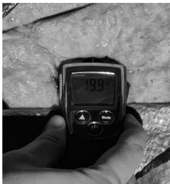
Figure 8 - Increased humidity of mineral wool at attic level
