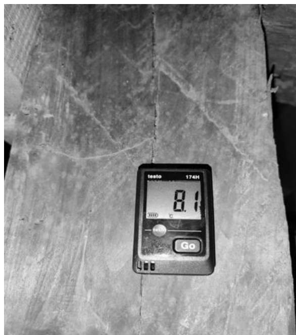
Figure 3 - Temperature measurement results using the Testo 174H recorder.
