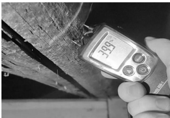
Figure 5 - The results of the moisture measurement of wooden rafters were performed using a Testo 606-1 moisture meter.
