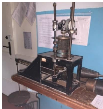
Figure 2 – Measurement of the load on the vibration damper with a limiter
