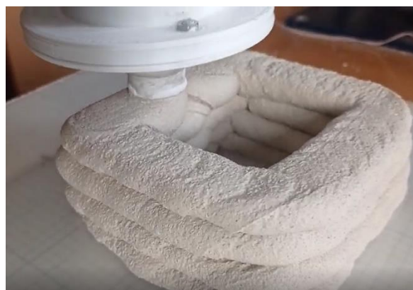
Figure 3 – The application of a layer of the concrete mixture onto the printing surface along a specified trajectory
