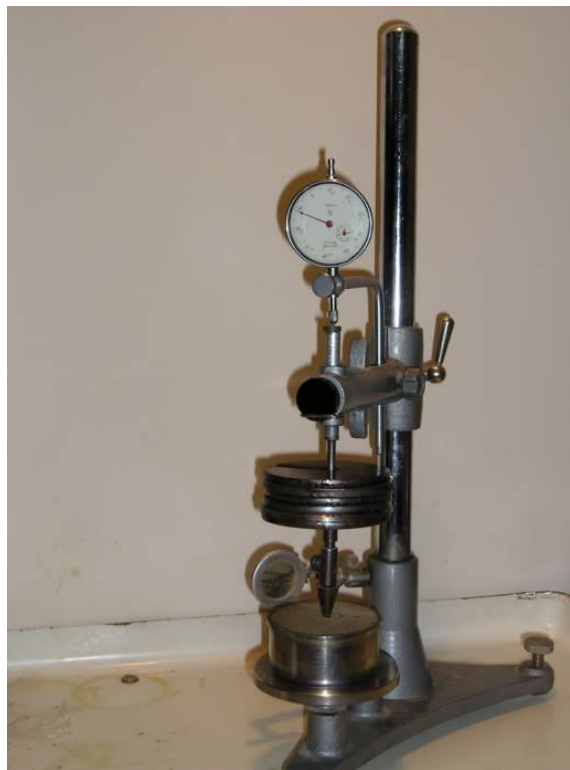
Figure 1 – Testing a clay rock sample with an advanced laboratory penetrometer
